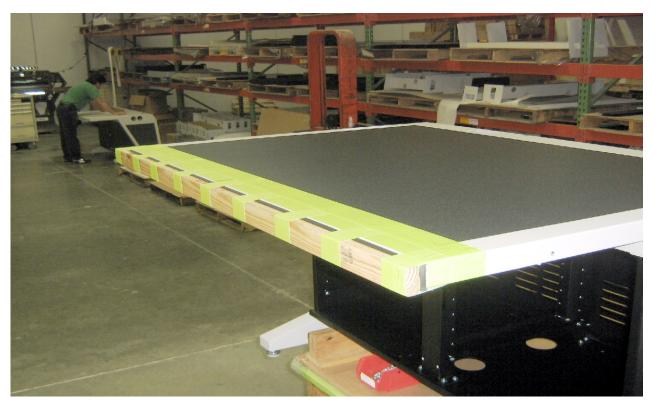
After removing existing Edgemold and applying beads of epoxy to upper and lower back side of Edgemold, secure to work surface with wood strips and tape
