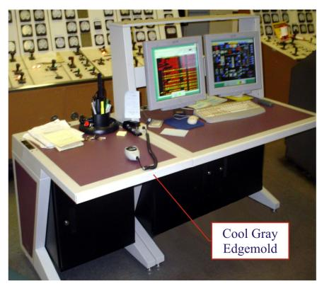
Edgemold Edgeguard prevents work surfaces from being chipped by rolling chairs, mobile printer tables, or file drawer modules on casters
