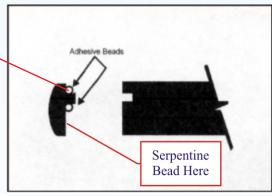
Install Edgemold in slots in console nose with rubber mallet and remove any adhesive with alcohol. Secure to front with straps of blue painters tape every 6 inches along the length of the Edgemold
