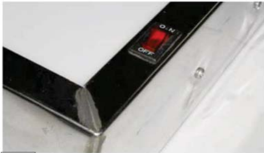
Simple On-Off Switch Impossible to create the desired luminance according to density of the developed x-ray film
